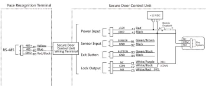
Figure 4-6 Wiring Secure Door Control Unit
