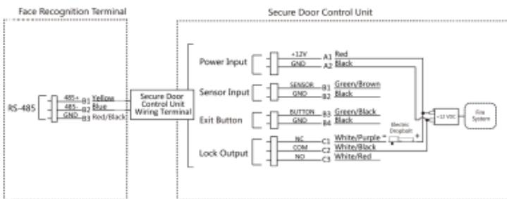
Figure 4-4 Wire Secure Door Control Unit
