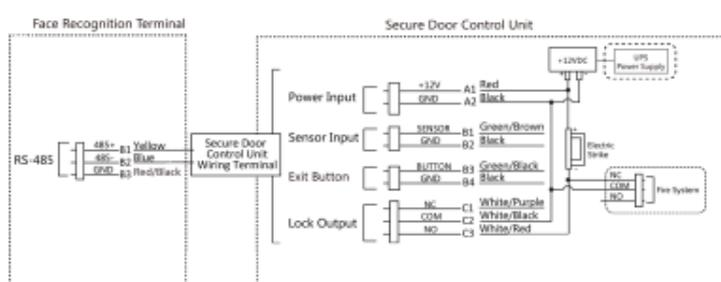
Figure 4-8 Wiring Diagram
