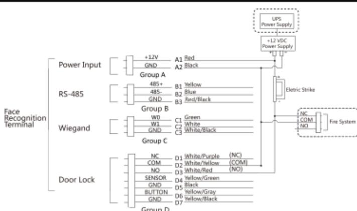
Figure 4-7 Device Wiring
