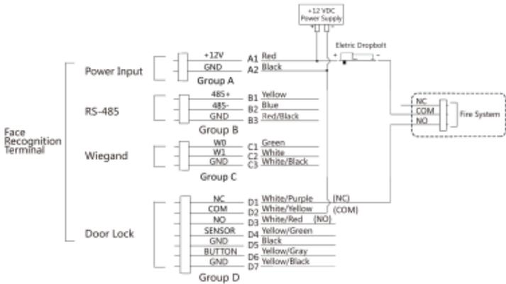
Figure 4-5 Wiring Device
