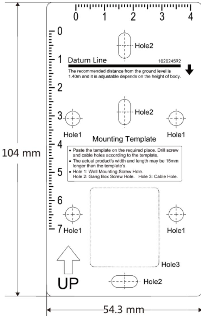
**Figure 3-7 Mounting Template**
