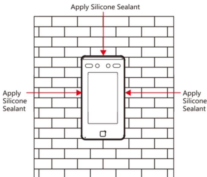
**Figure 3-6 Apply Silicone Sealant on the Side**
