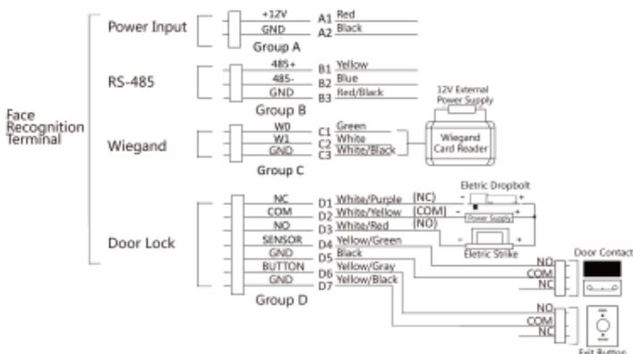
Figure 4-1 Device Wiring
