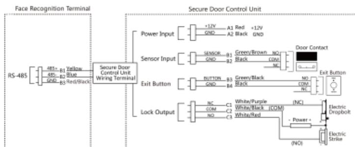
Figure 4-2 Secure Door Control Unit Wiring
