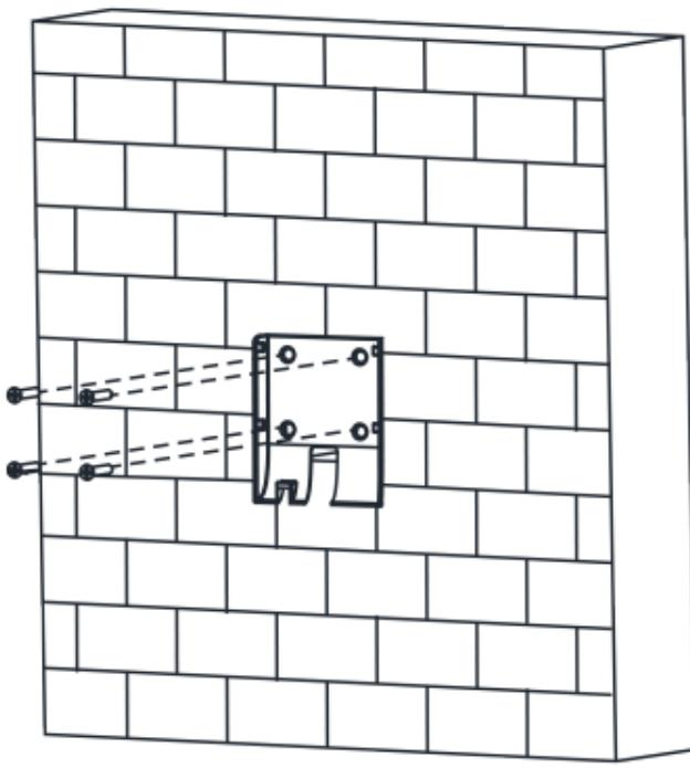
**Figure 3-8 Install Mounting Plate**
